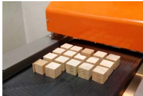
HSI, SPECIM, pixel size 625x625 \mu m, 900-2500 nm, 255 wavelength
