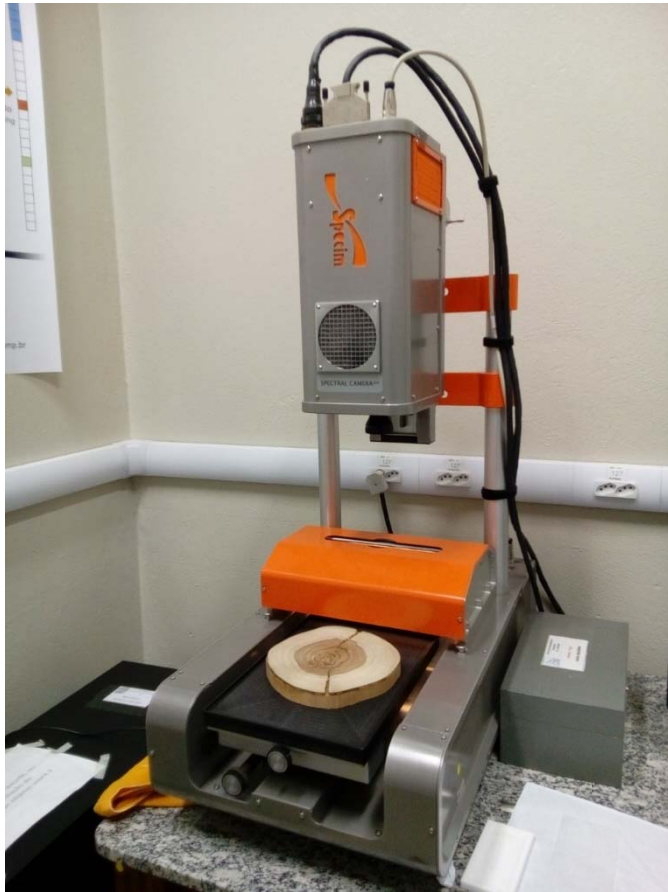
Image acquisition on wood disk Diameter disk 15 cm = 30 000 pixels = 30 000 spectra
