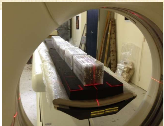
Scan of 1530 cores (15*17*6), Section of a bench of 17 core boxes
